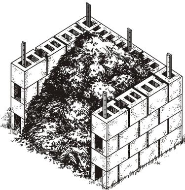
**Blocks or Bricks** - Just lay out the blocks or bricks without mortar. Leave spaces between the blocks or bricks to permit air to circulate. The best size is approximately 5 to 8 feet on a side and 3 to 4 feet high.
