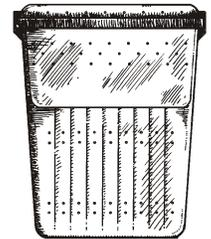
**What to Do** - Drill holes 4 to 6 inches apart all around your garbage can. You also need to drill holes into the bottom. (This allows for air movement and for excess water to drain off.) It is best to put 2 to 3 inches of straw or wood chips in the bottom to help it drain. Since a limited amount of air gets in, this system tends to work slower and the compost is wetter.
